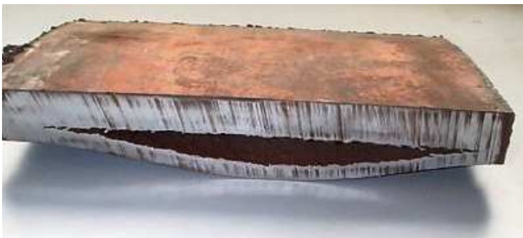
Specimen with huge hydrogen induced crack
