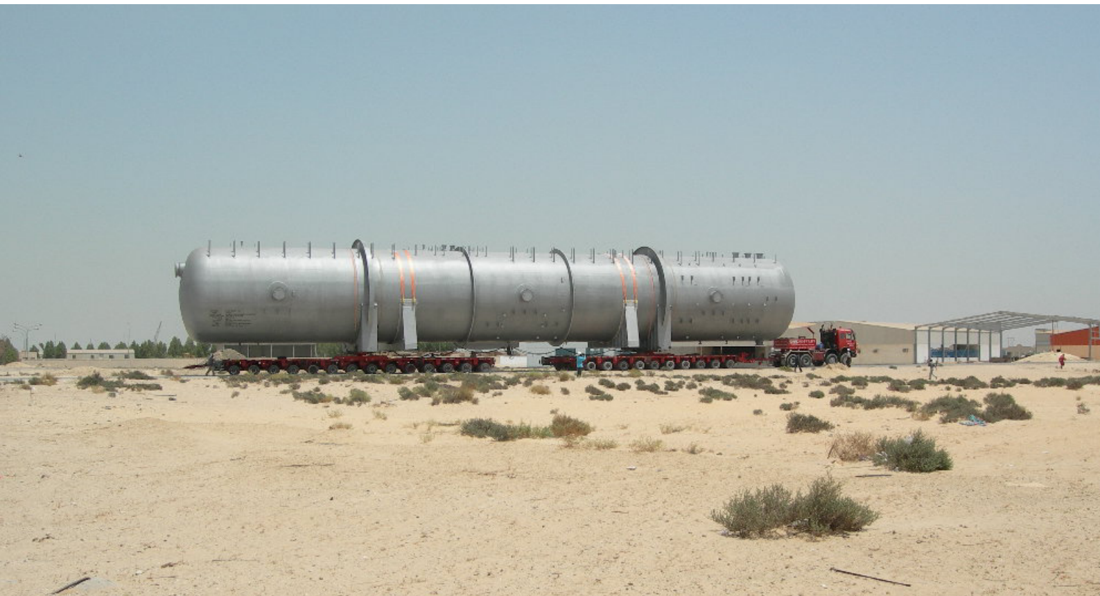
High Pressure Production Trap made of DICREST for the Haradh GOSP III project (courtesy of Gulf Engineering)
